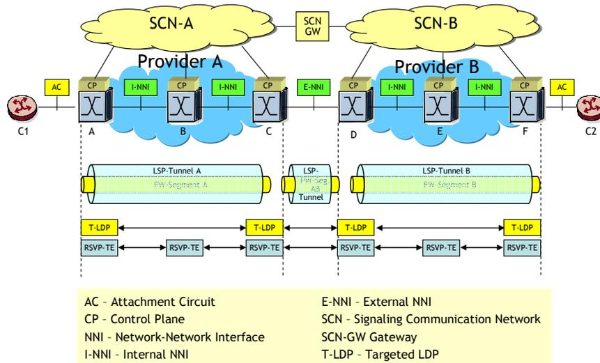
Figure 4: Control Plane View of a Multi-Segment Pseudowire
