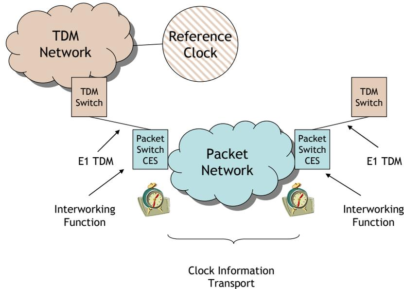
Figure 5: Clock Synchronization across a Packet Network
